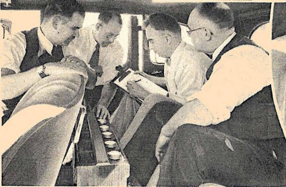
Experimental engineers are shown checking gas mileage after a test run. Each can holds an exact measure of various testing fuels.
