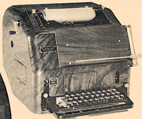
Above automatic telegraph typewriter both sends and receives. As sending machine it punches out tape which passes through transmitter to send electric impulses over wires.
