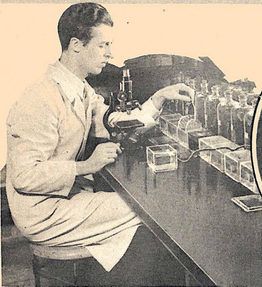
When staining slides in modern university laboratory, glass racks holding up to ten slides are transferred from one dyeing solution to another after proper period of immersion.
