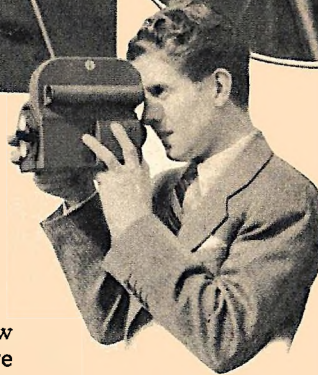
At left: Rudy Vallee speaks into mouthpiece at back of new "talkie" camera, recording on film running account of event being photographed. In circle: Close-up of camera and sound recorder on tripod, as used in recording sound effects. Weight of equipment is 20 pounds. With microphone, 110 volt a. c. power is used.
