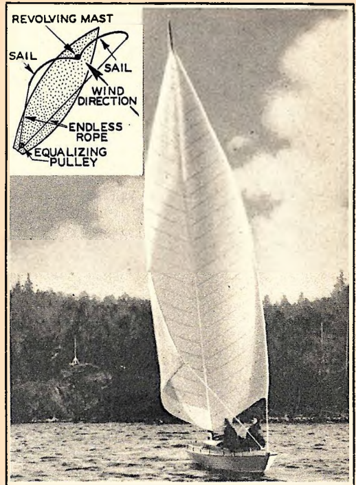
Fredrik Ljungstrom and two friends in a boat equipped with the new rigging. Upper left—Top view of rigging construction showing how it revolves to catch the wind.
