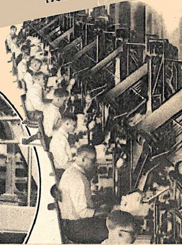
Linotype operators (right) hurriedly type-set the edited news in metal which is fitted into page forms for the presses (center). Papers then slide into news trucks (left) ready for delivery.
