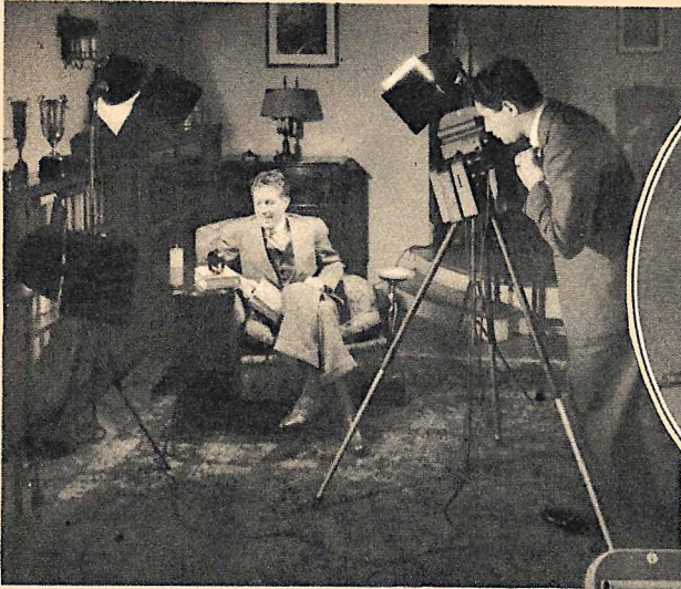
How "talkie" movies are made at home with actor speaking into microphone on end table at his right is shown above. At right—Photographer speaks into mouthpiece built into camera, his voice vibrating a thin metal diaphragm which is coupled to a tiny mirror. Light beam on mirror is reflected to sensitized edge of film to form sound track. Sound changes make fluctuations in film record.
