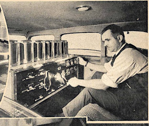
Above — Charles F. Becker is shown at the controls of the elaborate equipment used to test gas consumption under varying conditions. Left — Adjusting the heat control on a popular car prevents waste from imperfect fuel combustion.
