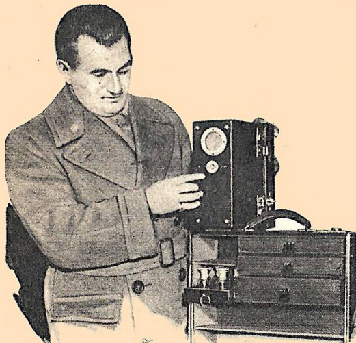
The inventor, H. Adler, with his talking bag unit designed to emit a warning cry when lifted by an unauthorized person.
