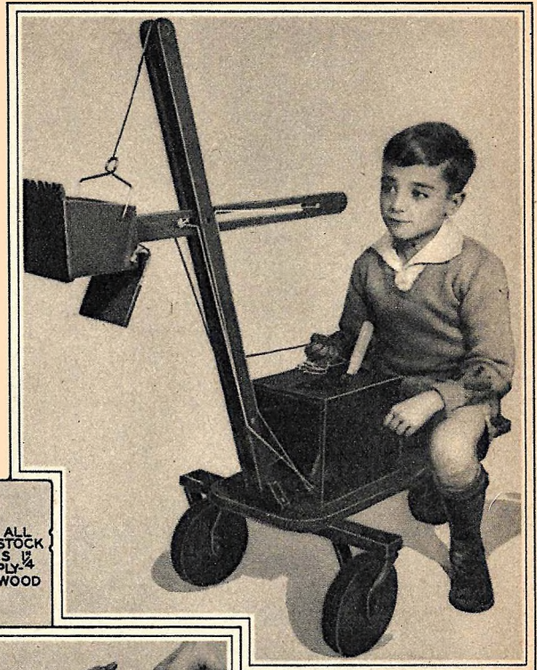
Here's how the completed shovel will appear. Bucket release cord is held in hand. Boom is at highest position here.
